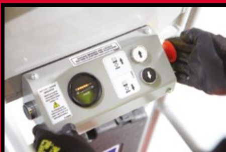
Both hands are safely in the basket when going up or down
