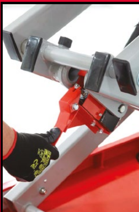
Easy access emergency lowering lever
