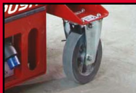
Auto brake prevents surfing
